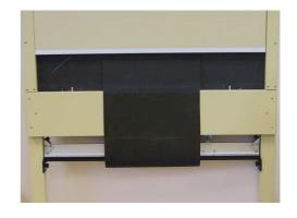
equipped with a black aiming area in 1mm black rubber. All external surfaces are painted in a off white colour, to achieve a comfortable aiming contrast and protection of the wood components.
