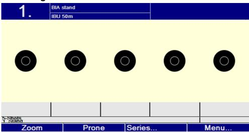
The shooter can switch between stand and prone position by pressing the B button. The LED indicatior on the target will light red when target is in stand position.
