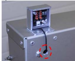
5. Plug the cable on the socket on the left of the motor controlling card inside the frame.
