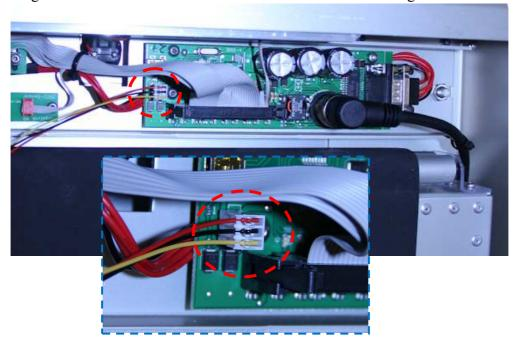
The plug is to be placed on the three pins to the left. There are two "taps" on the plug to hold it in place on the three pins behind.
